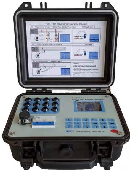
This equipment is used to help utility to analyze the basic information of end users, it can analyze and identify the supplied power of a network point (end user) come from which phase, feeder and transformer zone. The YCCI-9901 Phase and Feeder Identifier consists of two parts: Central Device (CD) and Line Device (LD). The CD will be connected to low voltage side of transformer, and LD will be carried by operator and installed to network points that will be analyzed.
