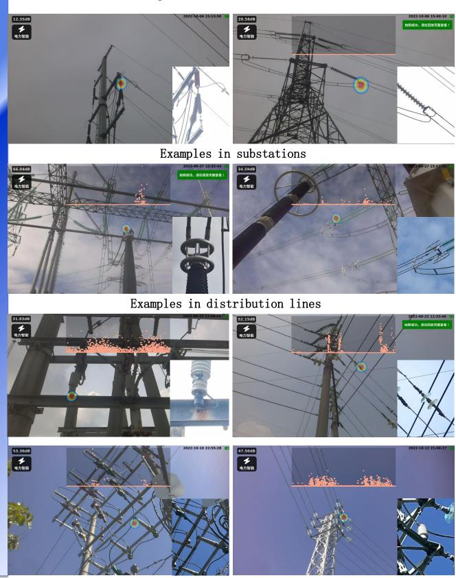
Focus Acoustic Camera, making sound and defects visible at a glance
